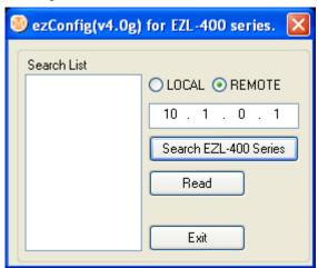
For the REMOTE SEARCH, user should select the [REMOTE] radio button in the initial window and input an IP address and press [Search EZL-400 Series], then the ezcfgmp searches EZL-410 with the IP address.
