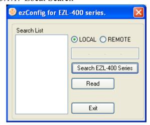
The LOCAL SEARCH method use UDP local broadcast with MAC address. So its benefit is that user can search EZL-410 although the user doesn't know the IP address of EZL-410. For LOCAL SEARCH, user should select [LOCAL] radio button and press [Search EZL-400 Series]. Then the ezcfgmp searches all EZL-410es in the local network. The found EZL-410es appear in the [Search List] window in form of its MAC address.
