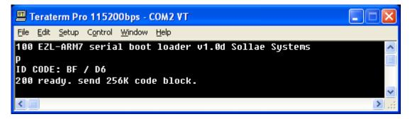
• In this time, if user send binary firmware that is supplied by us, then the following message is shown.
