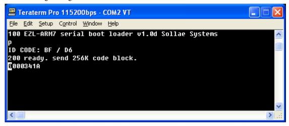
After firmware download is completed, EZL-410 checks its CRC. If there's no error, EZL-410 save the firmware its flash memory. And then it outputs the following messages.
